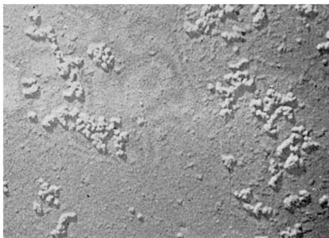
Fig. 9. Viscose D small gels. 23,375 \times actual.
